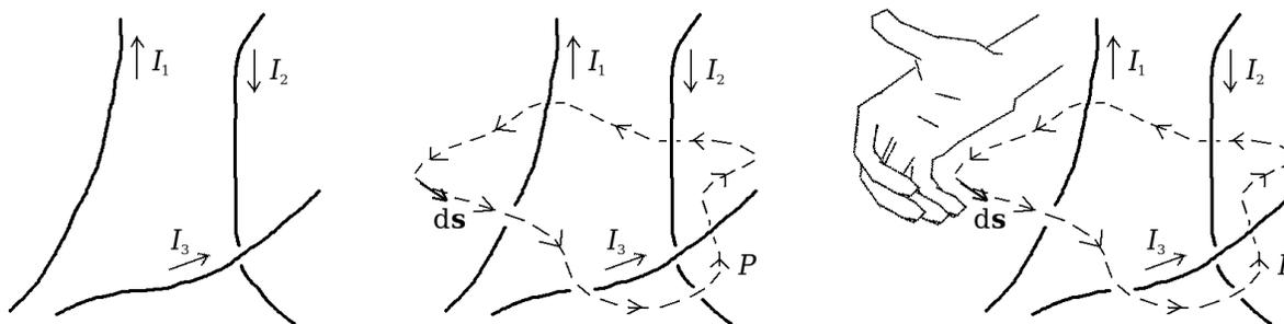
Figure 3: Loop/Threading Right Hand Rule, Monkey Style
